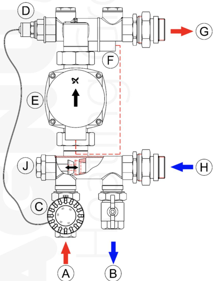
1. Connect the flow-side of the manifold to position G.
