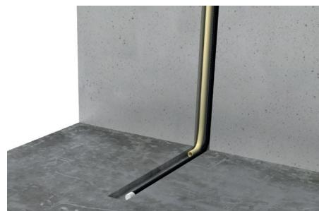
**TAKE CARE:** Never place the sensor in the vicinity of a (hidden) radiator pipe! Never install it passing under a heating cable!
