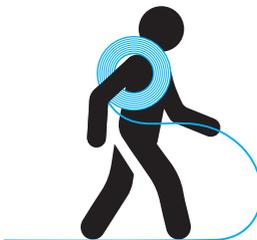
A floor heating tube is delivered as a roll and is therefore under tension. To prevent the heating tube lifting because of this tension, you need to unroll the coil in the opposite direction (see picture). This method lifts the tension for a large part.
